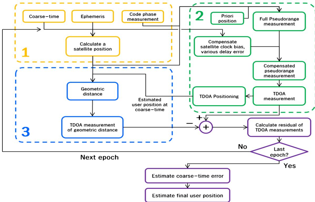
**Figure 3.** Flowchart of the proposed coarse-time positioning method
