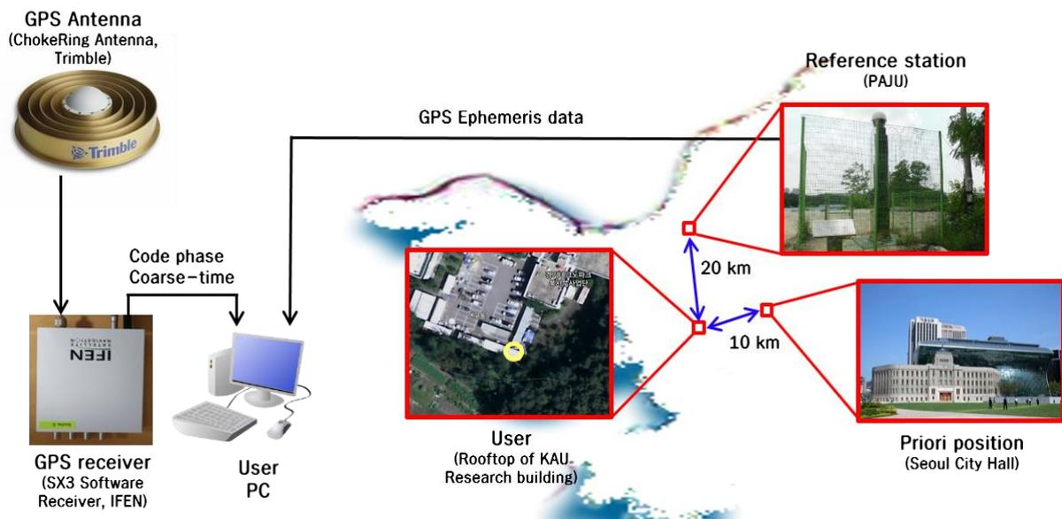
**Figure 4.** Experiment configuration
