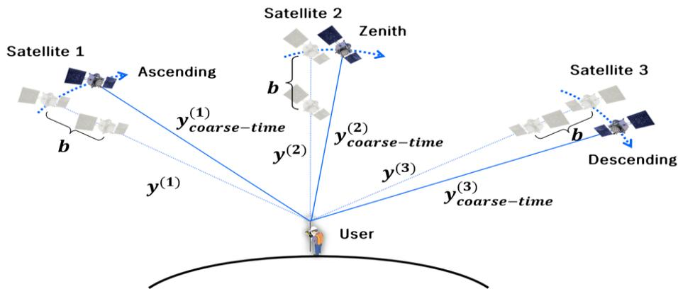
**Figure 2.** The effect of coarse-time error(Van, 2009)
