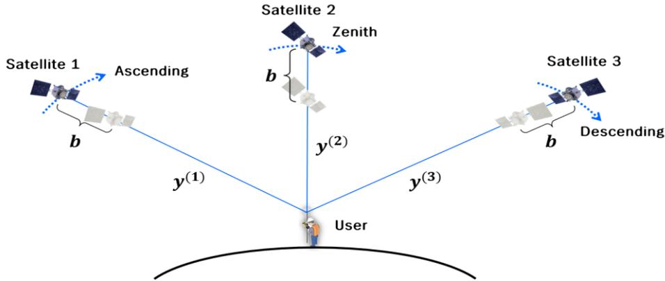
**Figure 1.** The effect of receiver clock bias(Van, 2009)
