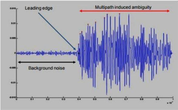
**Figure 3: Signal received by a UWB receiver kept in a cluttered environment. (After White paper: Time Domain P410 UWB)**
