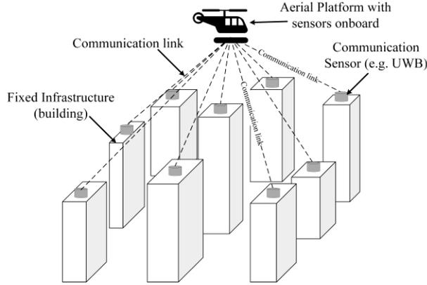
**Figure 4: A Cooperative P2I localization system (After Goel et al. 2016b).**
