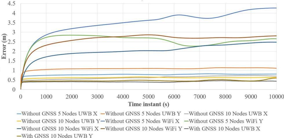
Figure 7: RMS error in trajectory of platform along X and Y directions. It is assumed that GNSS is not present and either UWB or Wi-Fi aids the platform in localization.
