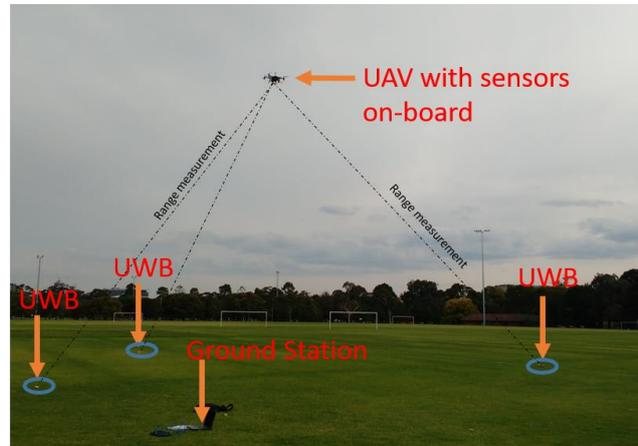
**Figure 9: Experimental setup of cooperative P2I localization.**
