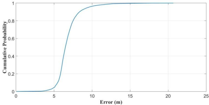
**Figure 14: CDF plot of error in UAV location.**
