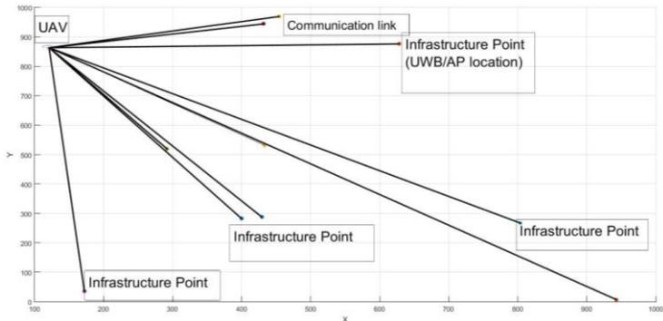
Figure 6: An example of a cooperative network with 10 infrastructure nodes (Plan view).
