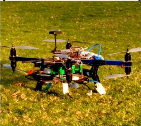
**Figure 8: Prototype cooperative localization UAV platform. UWB, GNSS and INS along with raspberry Pi is integrated on UAV.**
