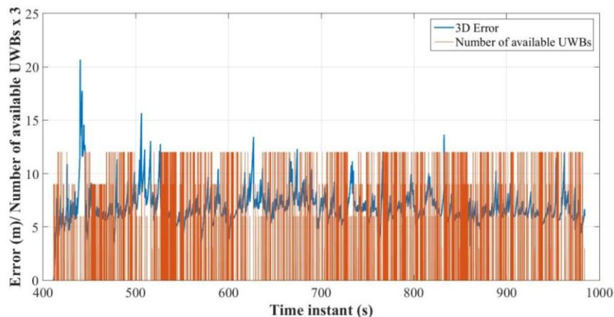
**Figure 12: Error plot (w.r.t GNSS) of UAV location with UWB availability overlaid.**
