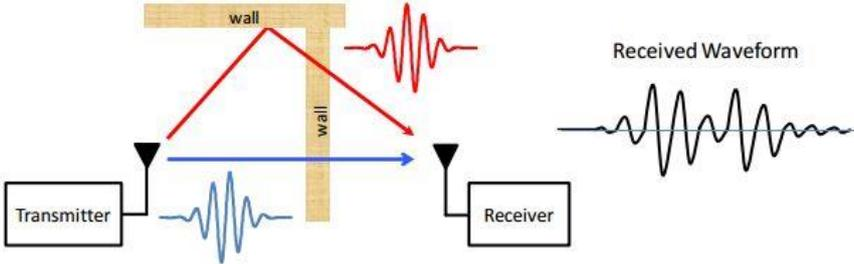
**Figure 2: Multipath in a cluttered environment. The transmitted pulse is shown in blue, reflected pulse in red and received pulse in black. (After White paper: Time Domain P410 UWB).**
