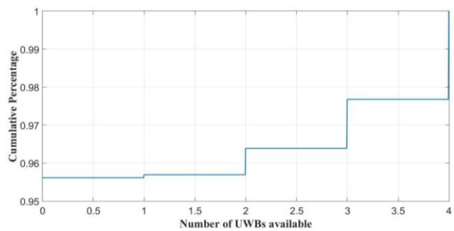
**Figure 11: Plot of availability of UWB measurements during the localization experiment.**
