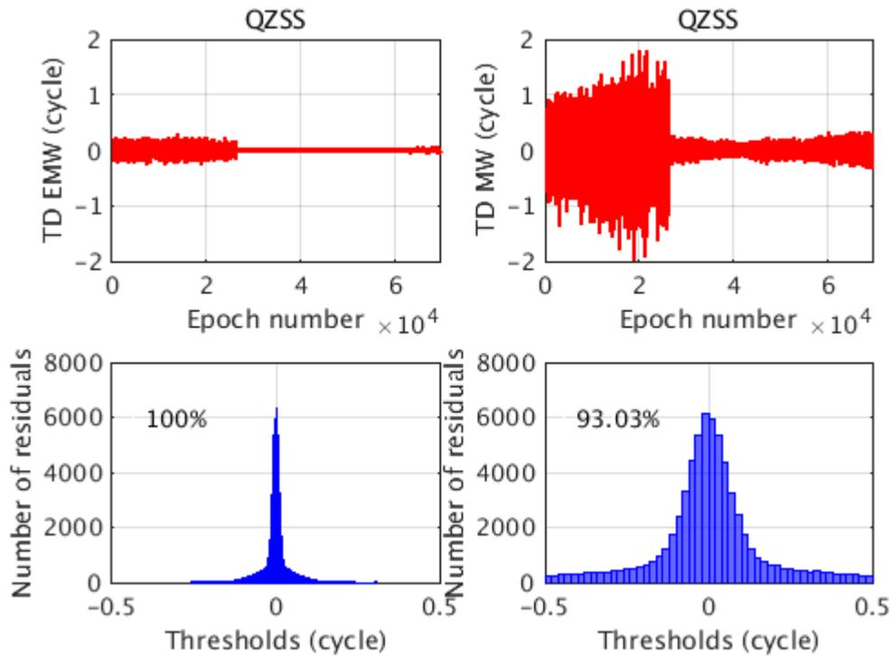
**Figure 5.** QZSS TD EMW and TD MW noise analysis
