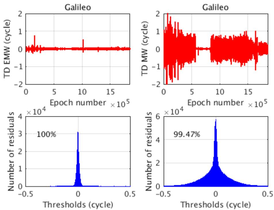
**Figure 4.** Galileo TD EMW and TD MW noise analysis
