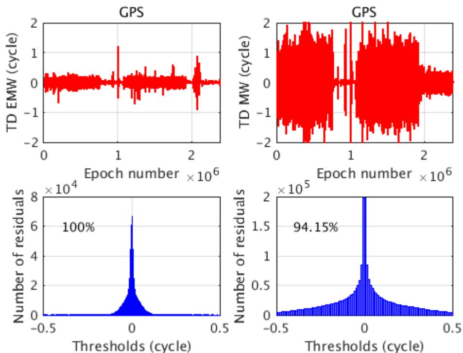
**Figure 2.** GPS TD EMW and TD MW noise analysis
