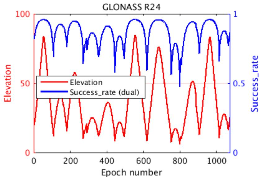
**Figure 8.** ILS success-rate versus satellite elevation for GLONASS (FDMA)
