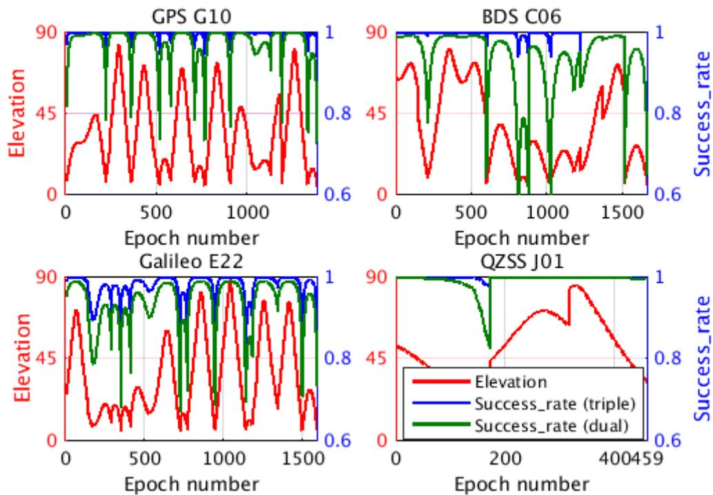
**Figure 7.** ILS success-rates versus satellite elevations for CDMA based satellite systems
