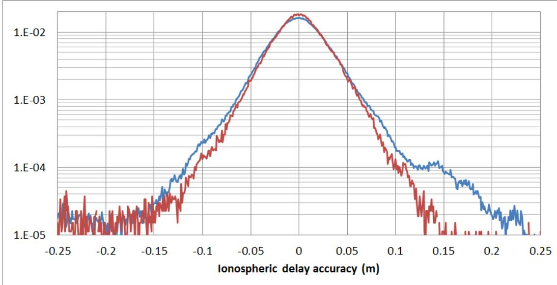
**Figure 2.** Differences between measured and interpolated ionospheric delay estimates. The ionospheric delay estimates were computed based on CLK91 (red) and MADOCA (blue) products.
