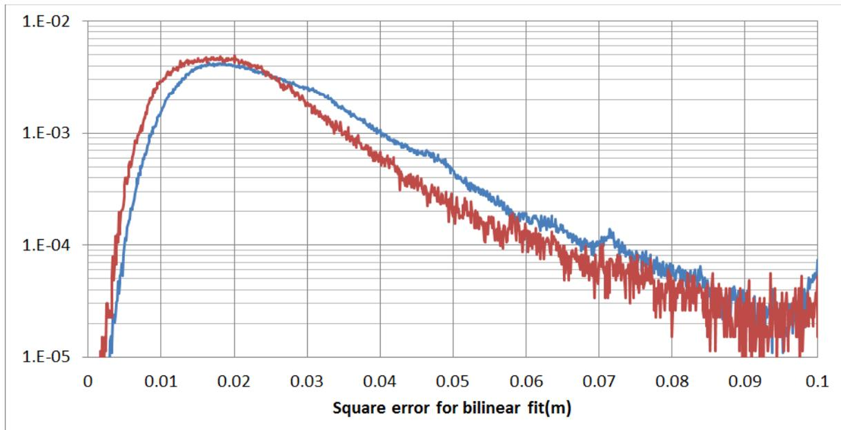
**Figure 3.** Mean Square errors of bilinear fit for ionospheric delays. Ionospheric delays were calculated based in CLK91 (blue) and MADOCA (red) products.
