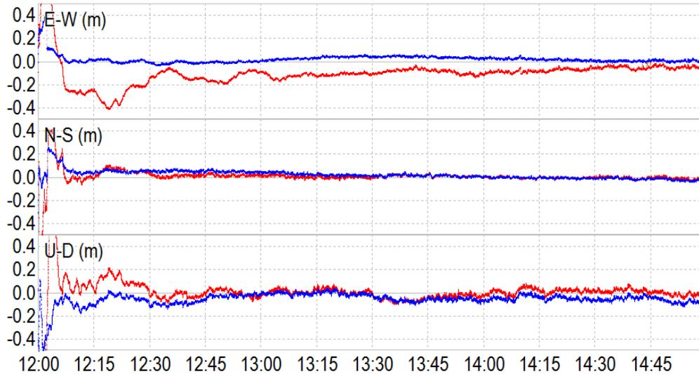
**Figure 5.** Example of PPP (red) and PPP+Ion (blue) positioning solutions using MADOCA products.
