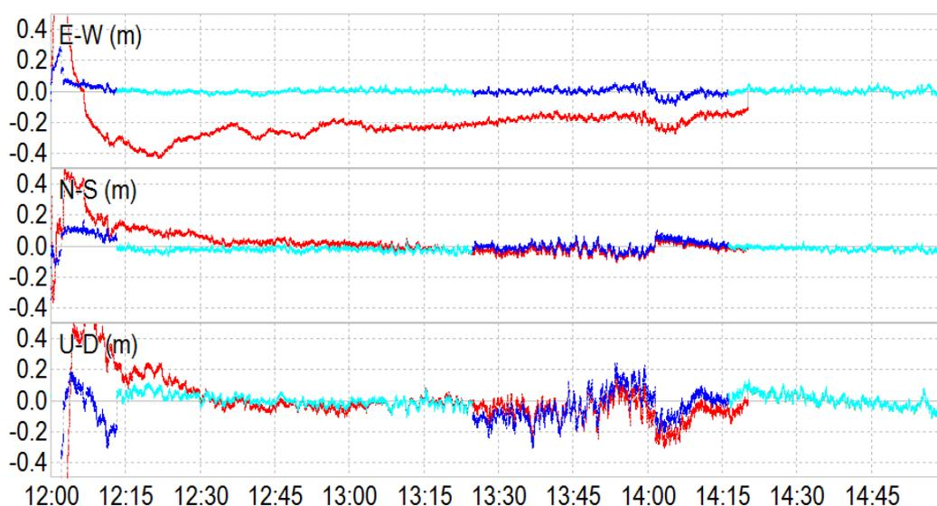
**Figure 4.** Example of PPP (red) and PPP+Ion (blue) positioning solutions using CLK91 products. Dark line corresponds to unfixed solutions, light line corresponds to ambiguity fixed solutions.
