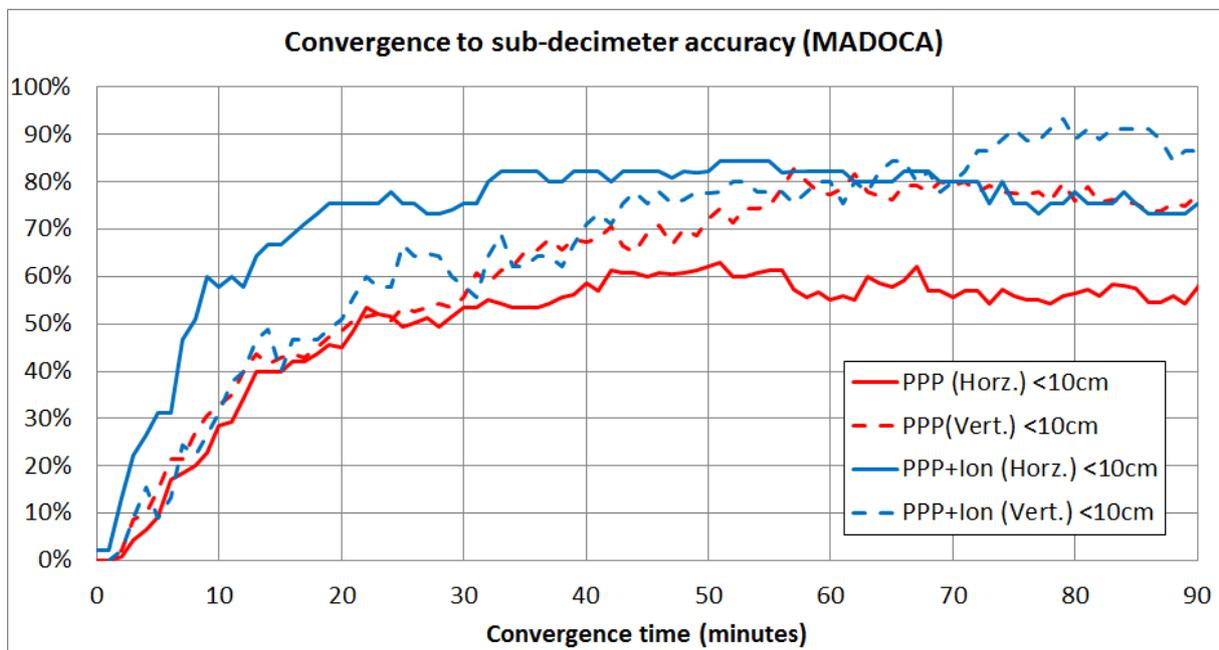
**Figure 8.** Percentage of solutions with Vertical (dashed) and Horizontal (solid) RMS errors below 10cm for different times of convergence. Red lines represent MADOCA based PPP solutions, blue lines represent PPP+Ion solutions.
