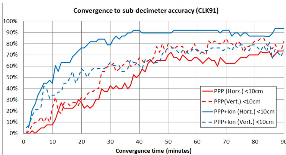
**Figure 6.** Percentage of solutions with Vertical (dashed) and Horizontal (solid) RMS errors below 10 cm for different times of convergence. Red lines represent CLK91 based PPP solutions; blue lines represent CLK91 based PPP+Ion solutions.
